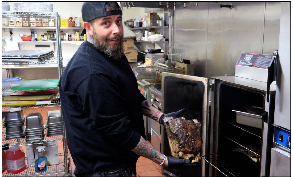
The Southern Pride appliance now used at Butcher Block BBQ replaces a traditional smoker that produces excessive smoke. The appliance also does not use an open flame and has a self-timer and a continuous fan to ensure all of the meat is cooked evenly. Photo credit: Taylor Hillo
