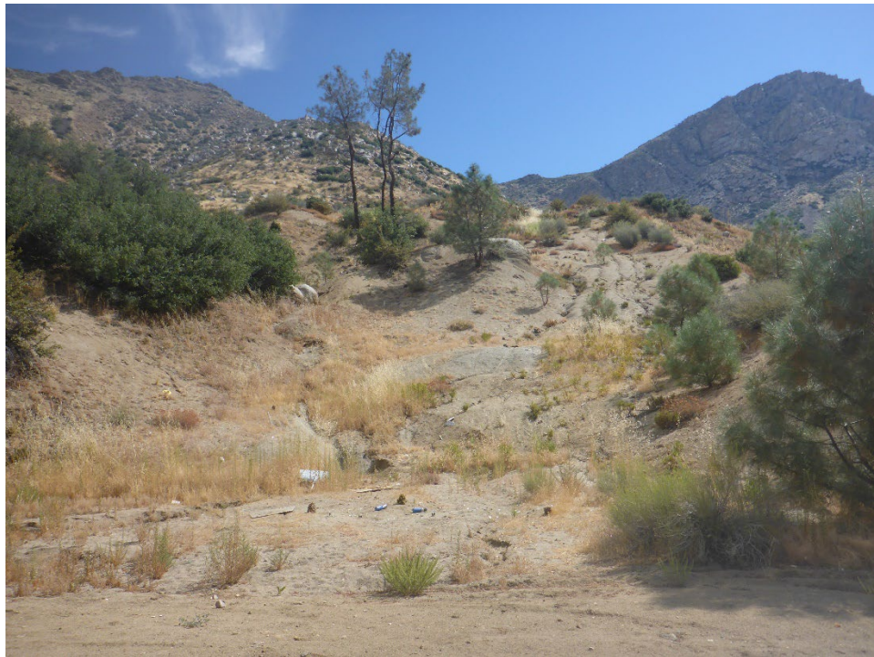
Figure A-8. Minor surface rilling cut into native decomposed granite hillslope at Tunnel 4/5 Spoil Site. Material potentially historical tunnel spoil material; sediment delivery captured by Tunnels 5-8A Access Road and spoil pile pad.
