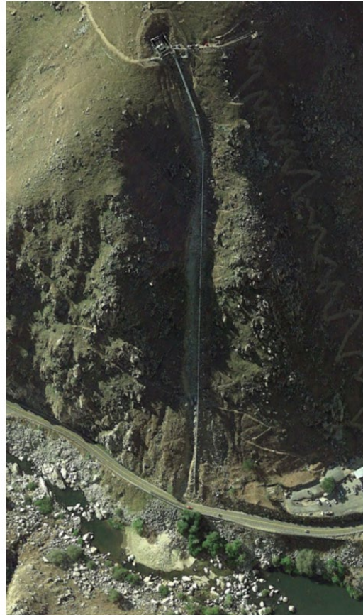
Photo A-22. KR1 Penstock Erosion and Sediment Deposition in the Kern River Channel After the August 20, 2013, Forebay Spill Event (Google Earth Image, Date: 4/15/2014)
