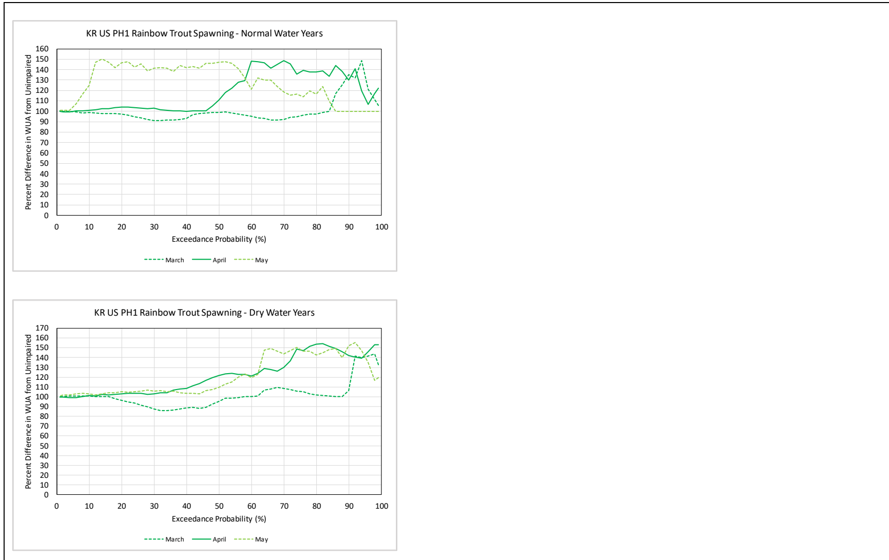
Figure B8.4-14. Kaweah River Downstream of East Fork Kaweah Confluence and Upstream of Kaweah No. 1 Powerhouse Rainbow Adult Spawning Percent of Unimpaired Habitat Exceedance Plots (1994-2018) for Normal (top) and Dry Water Year Types (bottom) using Proposed Action Minimum Instream Flows
