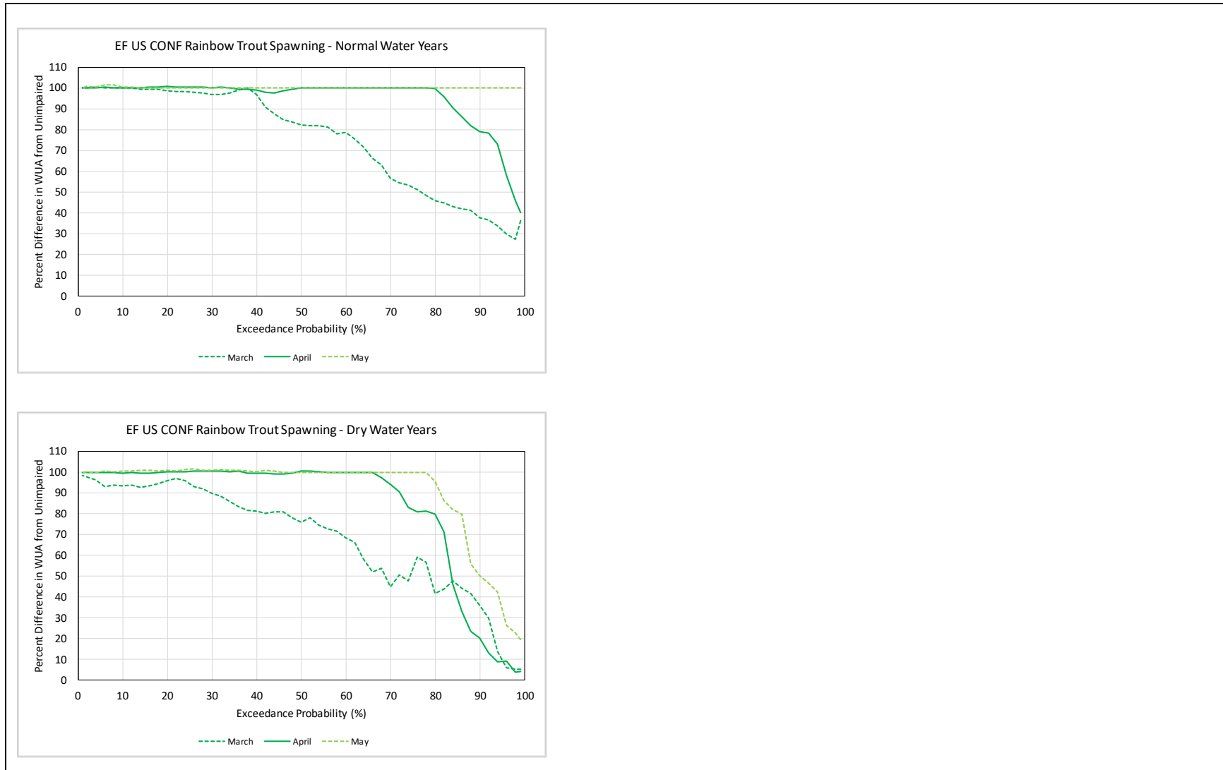
Figure B8.4-28. East Fork Kaweah River Upstream of the Confluence with Kaweah River Rainbow Adult Spawning Percent of Unimpaired Habitat Exceedance Plots (1994-2018) for Normal (top) and Dry Water Year Types (bottom) using Proposed Action Minimum Instream Flows
