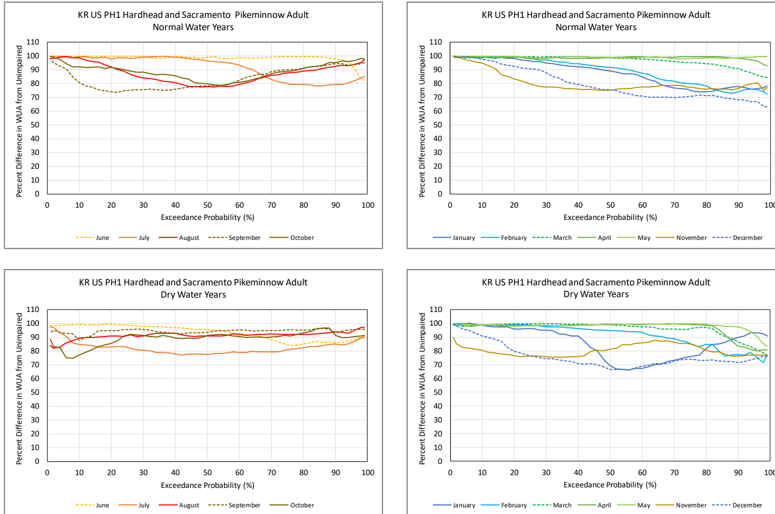
Figure AQ 1-15. Kaweah River Downstream of East Fork Kaweah Confluence and Upstream of Kaweah No. 1 Powerhouse Hardhead and Sacramento Pikeminnow Adult Habitat Percent of Unimpaired Exceedance Plots for Normal and Dry Water Years.
