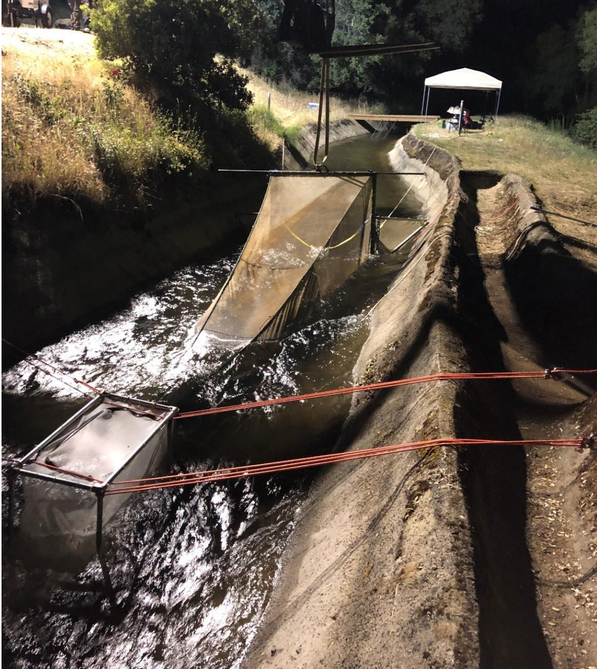
Figure AQ 9-15. Fyke net with wing walls and live car set up at Kaweah No. 2 Flowline.
