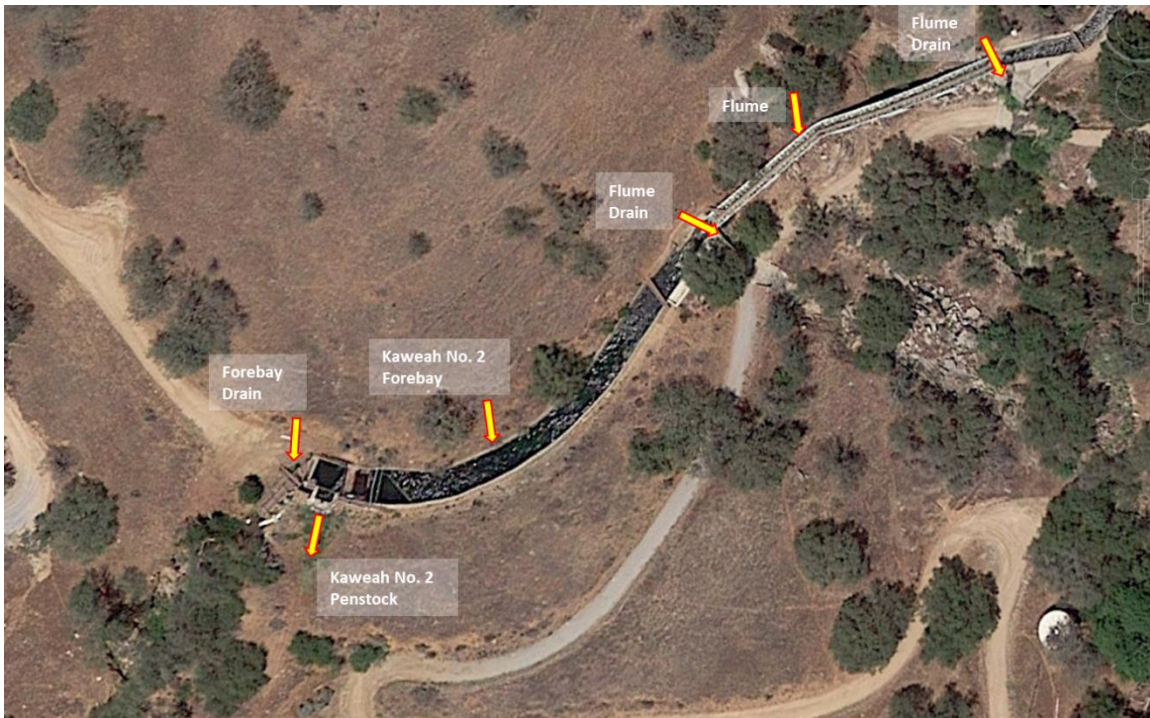
Figure AQ 9-10. Kaweah No. 2 Forebay, Flume and Penstock, and Drains.
