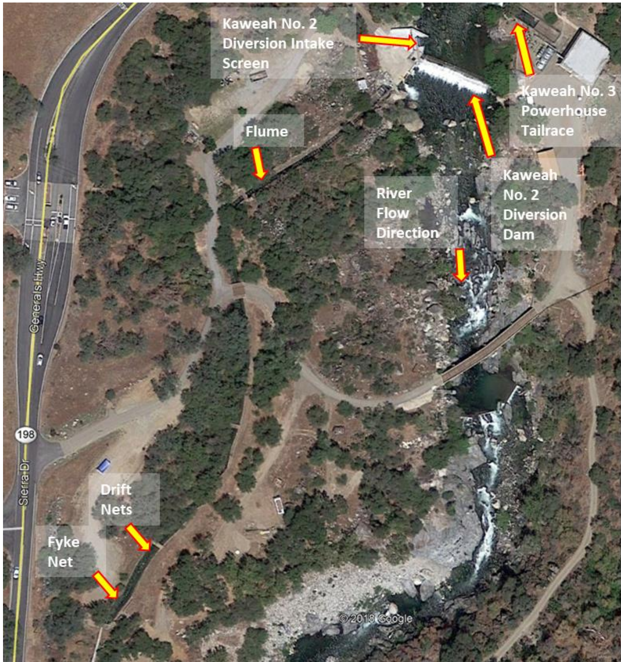
Figure AQ 9-14. Kaweah No. 2 Flowline fyke net and drift net sampling location.
