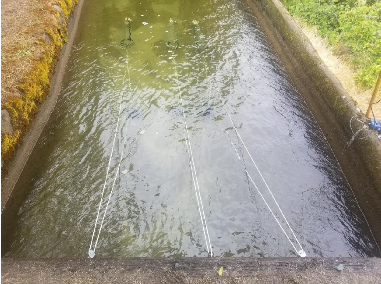
Figure AQ 9-18. Three drift nets with 6-inch diameter opening deployed at a wooden bridge immediately upstream of the Kaweah No. 3 Forebay.
