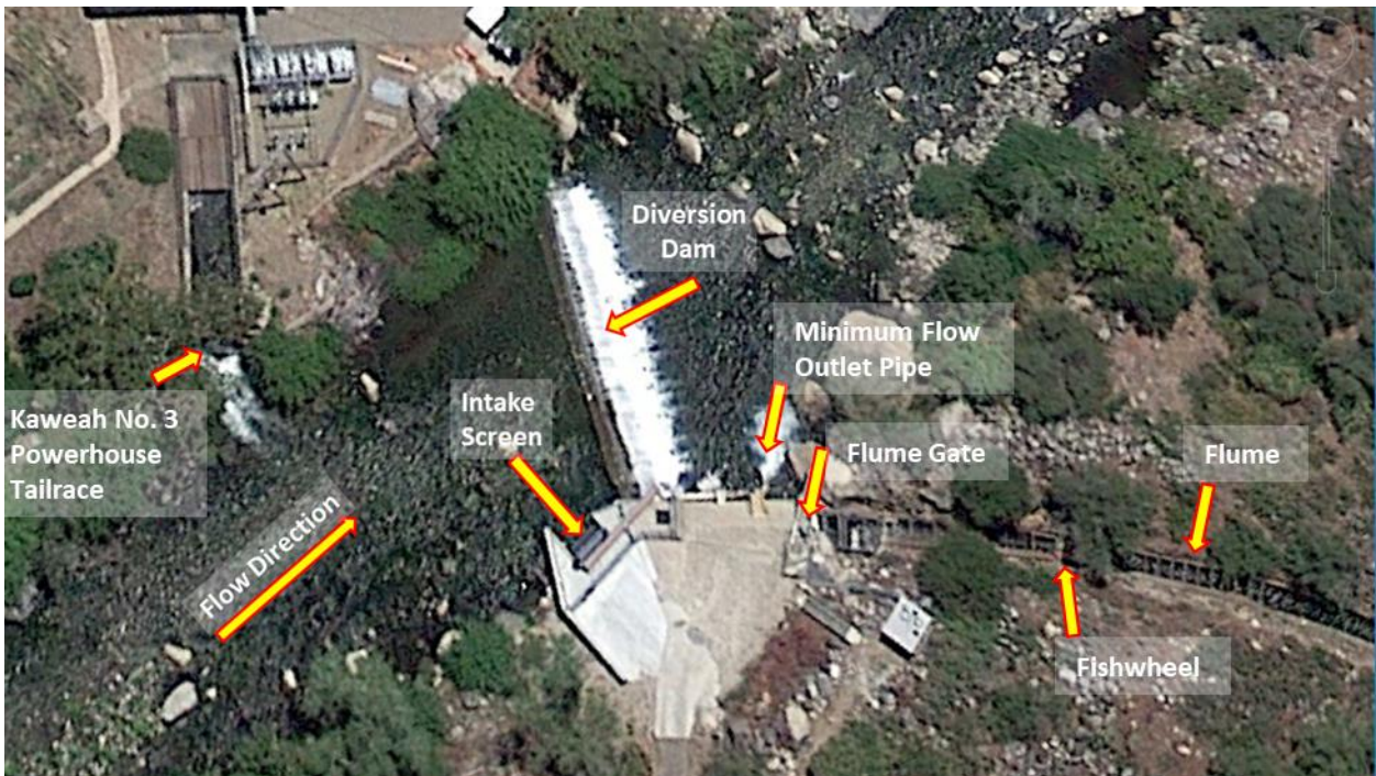
Figure AQ 9-6. Aerial view of the Kaweah No. 2 Flowline Intake with key feature labeled.
