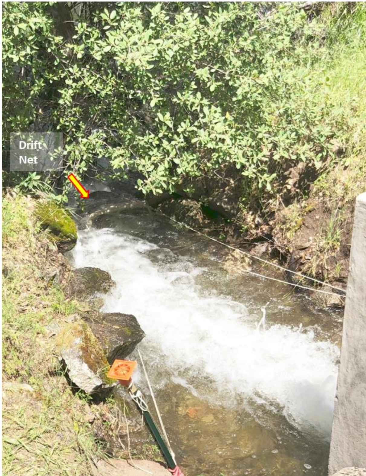
Figure AQ 9-13. Drift net with 12-inch by 17-inch rectangular opening deployed in Kaweah No. 1 Flowline immediately downstream of the flowline sampling section where the flowline water was returned back to the East Fork Kaweah River. Flow approximately 6.2 cfs.
