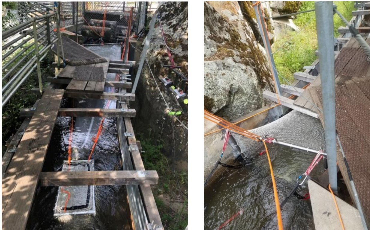
Figure AQ 9-12. Fyke net and live car set up at Kaweah No. 1 Flowline (left image looking upstream, right image looking downstream). Flow approximately 7.2 cfs.
