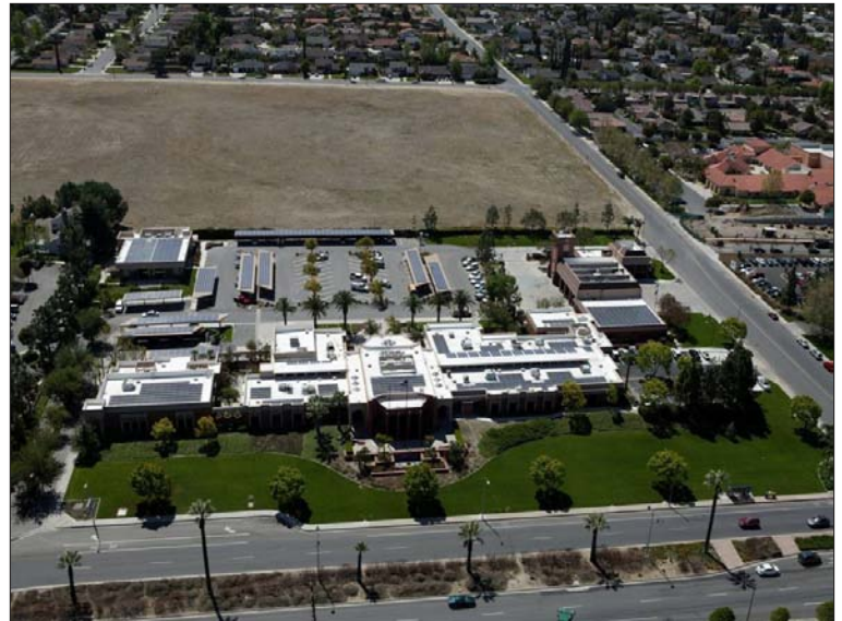
The City of Loma Linda shows its commitment to renewable energy with solar energy systems on its Civic Center that generate about 282 kW.
