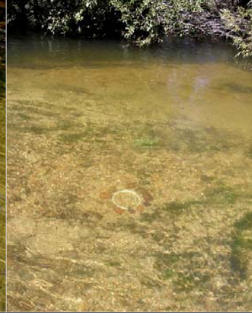
Run 1 - Lower monitoring site After 425 cfs Visible PT was uncovered; other one is still buried in the background.
